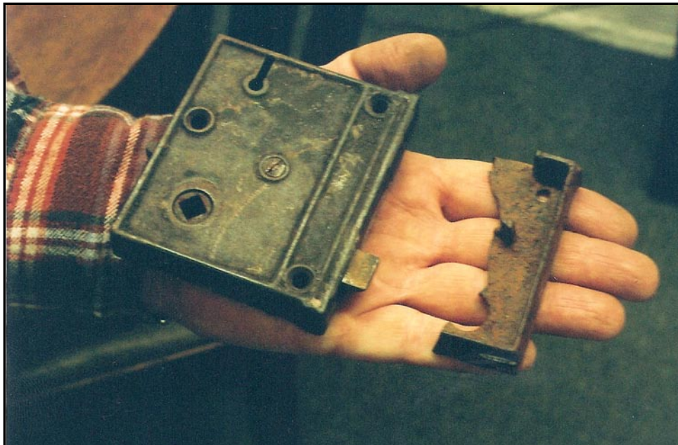
Figure 423. Owner Wes Creager of Briarwood Antiques and Collectibles in San Jose, CA, sells this same type of door lock that he believes “dates back to the Civil War.” Notice its latch (in middle foreground above) that looks like a little tongue protruding. The cast iron piece (above right) is specimen 320-433b found at the Hi Good Cabin site, with 3 1/4” length. It is a part of the back plate side, the part that goes with the end that has the hole (with square opening) for the hand knob and connecting inside and outside hand knobs.
