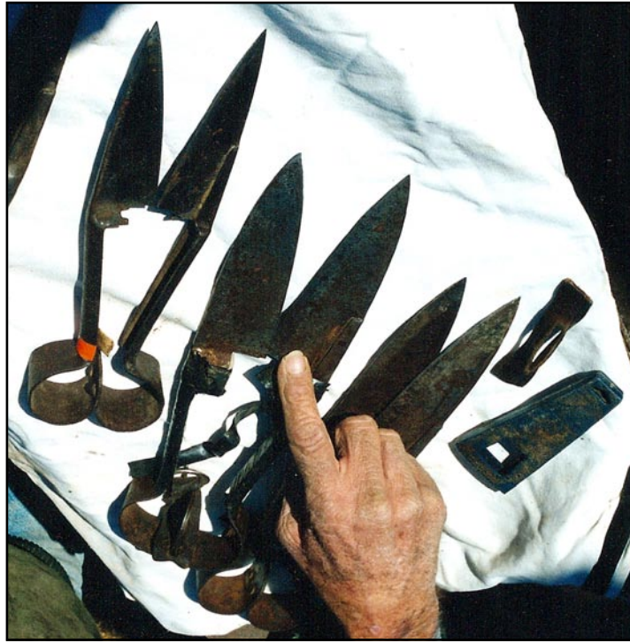
Figure 402. Jack Haslem points to blunt tip sheep shears (middle pair) as contrasted to sharply tipped sheep shears (left and right). In the photos' right side, two types of "keepers" are displayed. Keepers "keep" the sheep hand shear blades together to protect the blades. All three pairs are double springs. The blunt tip pair of Burgon & Ball sheep shears (below) belonged to a fellow named Irving Beard from Fruita, Colorado, of Mesa County, who was a professional sheep shearer.
