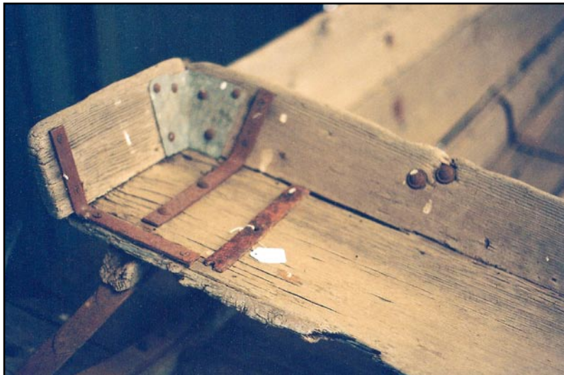
Figure 312. Wagon's metal reinforcement strap (320-560), with white tag in photo (left), is a near match with this wagon's metal reinforcement strip, used to help hold together its buckboard seat. This old buckboard wagon is preserved at the old Patrick's Ranch, the Northgraves Mansion, Durham, California, for whom Chico's Far West Heritage Association is the steward. Photo by author.
