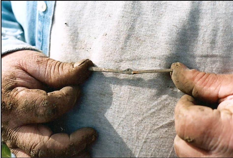
Figure 425. “This piece (specimen 320-119) is 3.5” x 1/8” x 1/16.” It is conceivably a manual pivoting piece of a door rim mounted lock, which always is mounted on the “inside” of the door for locking the lock without a key. This piece might go with a series of other internal pieces which, when taken together, makes the bolt to work in the lock or unlock positions.” —Cliff Moffitt, Locksmith Consultant
